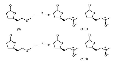
a) Ti(OiPr)<sub>4</sub>, (-)-diethyl tartrate, 'BuOOH, CH<sub>2</sub>Cl<sub>2</sub> (25%);
